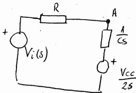
$$\begin{aligned} \text{donde } V_i(s) &= \mathcal{L}\{-V_{cc} \cdot u(t)\} = \\ &= -V_{cc} \cdot \mathcal{L}\{u(t)\} = -\frac{V_{cc}}{s} \end{aligned}$$
