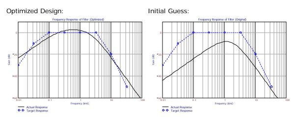
Note that we needed to specify several points within the passband in order to force Mathcad's optimizer to keep the mid-band gain down. Without these extra points the "skirts" become better matched and the mid-band gain became too large, as shown below:
