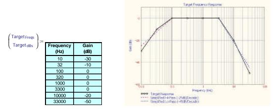
As can be deduced by inspecting the table, we wish our filter to be "flat" from 100 to 3300 Hz, and have approximately 25dB/decade below and 45db/decade above that range. Obviously, real world filters have slopes of 20 and 40 dB/decade, so, our optimized filter will be "close, but no gold cigar". There is NO way to exactly provide this shape, but, perhaps we can create a filter that is "good enough".
