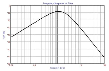
Next, we wish to optimize the circuit so that it performs to some desired response. This desired response (aka goal function) might be taken from a customer requirements document, or from a specification created by the system designer. For this example, we are going to fill a pair of vectors with Frequency/dB target points that we would like our filter's response to pass through. We can make use of an embedded Excel table to make the data-entry easy and professional looking:
