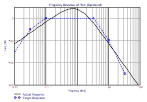
In fact, with two minor modifications we can provide additional constraints to make some target points more important than others:
