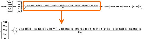
After collecting on terms  $Vio,\ Ib,\ and\ Io\ the\ V_{Out}$  function declaration changes to:
