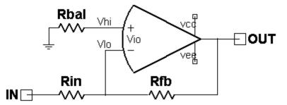
Derive the nodal equations, presuming input currents are zero (ideal op-amp), but provide a term for the input offset voltage (**Vio**):
