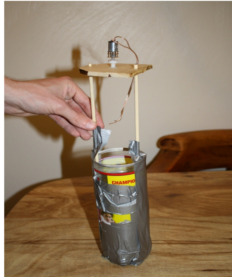
Figure 2. The Motor shaft is connected to the racquet-ball container shell through 4 dowel rods
