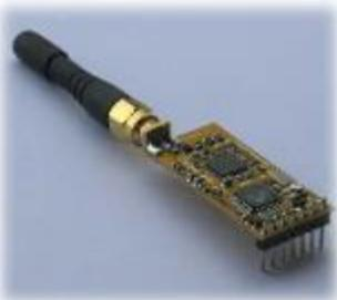
In the Arduino CanSat kit we are using APC220 which is a transceiver, with a highly versatile low power radio solution that is easy to setup and integrate into any project requiring a wireless RF link.
