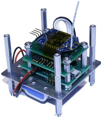
Be careful with aluminum standoffs and other aluminum hardware. The thread side can be broken off if tightened too much.
