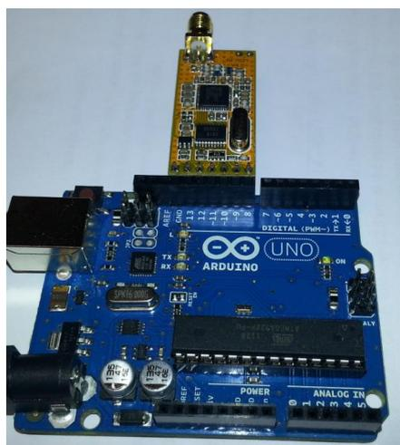
Figur 12: Connecting the transceiver to the Arduino UNO board
