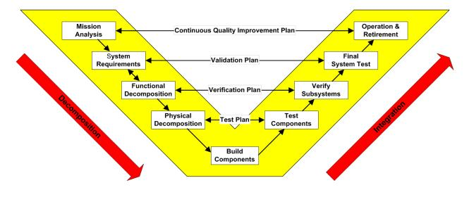
The design downstroke and the manufacturing upstroke
