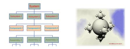
The systems engineering process is applied at levels of greater and greater detail.
