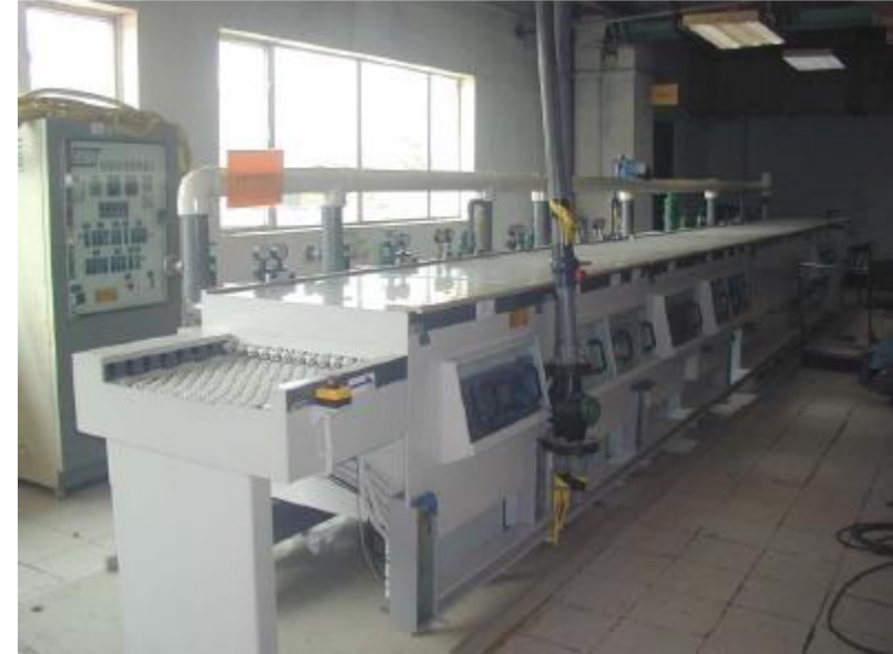
Conveyorized Horizontal OSP and Pre-Flux Line
