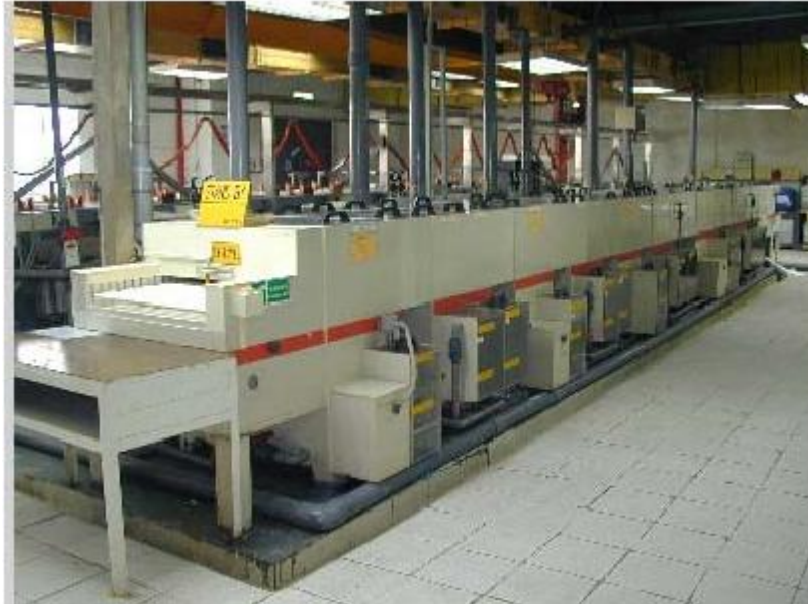
Conveyorized Horizontal OSP and Pre-Flux Line
