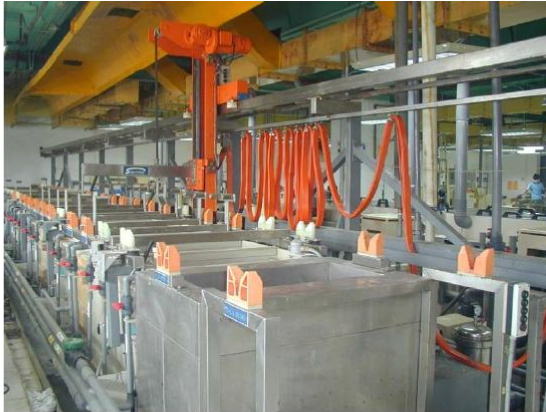
Automated Immersion Tin Plating Line
