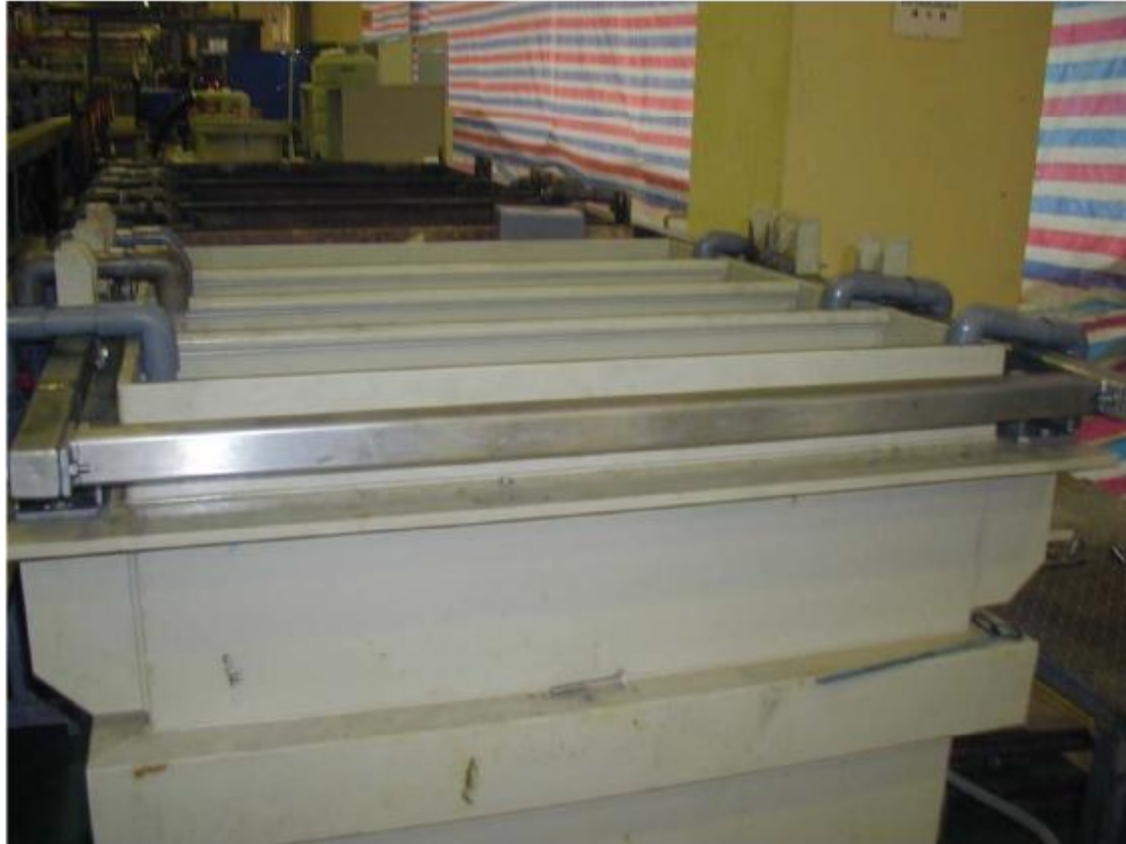
Manual Tin-Lead Plating Line
