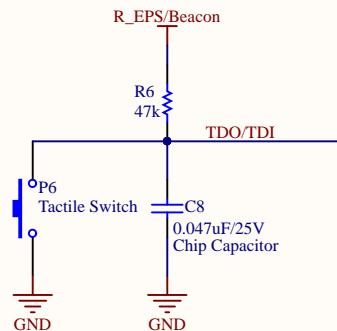
The reset system has a switch, a 47k resistor and a 47 nF capacitor. This reset affects to TDO via, which comes from the JP1 connector. Its voltage is provided by the R\_EPS/Beacon signal.
