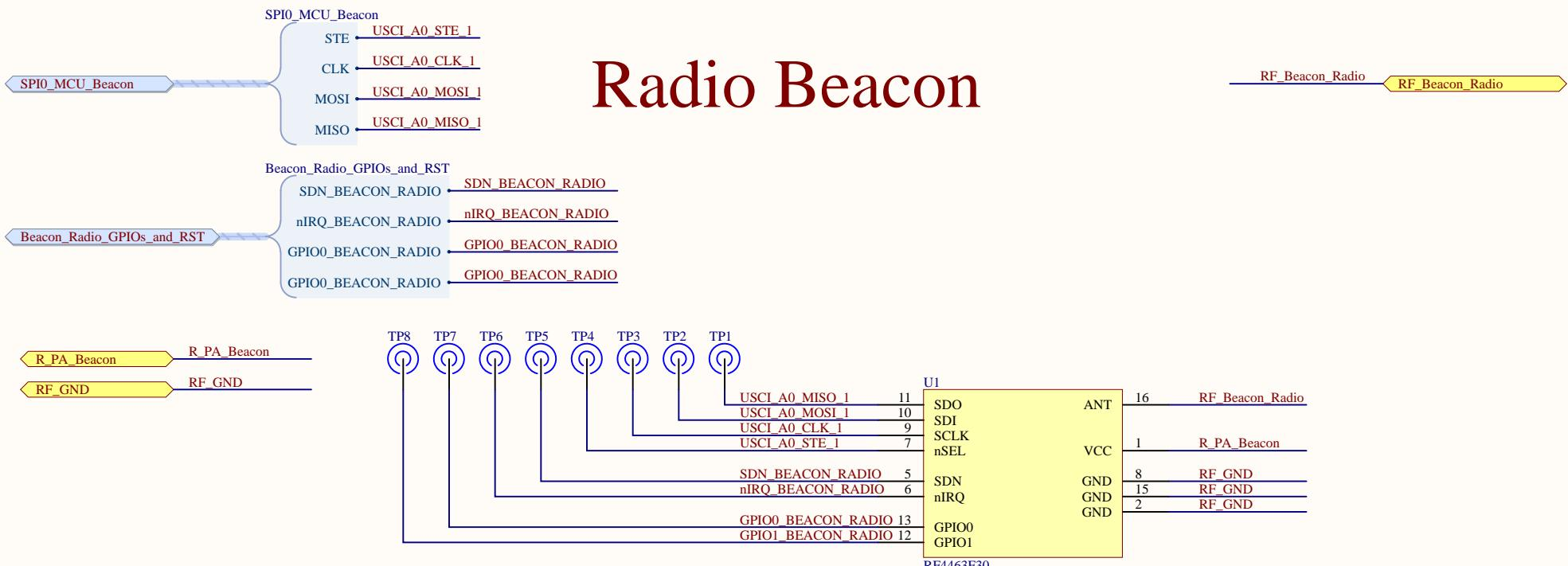
This is the radio beacon schematic. We are using a RF4463F30 module. Different signals can be seen (two signal harnesses). Those different signals are ruted to different test points.
