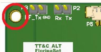
The "Screw\_Mx" (with x content between 1 and 4) are referred to the holes found in the corners of the PCB, which are connected to ground. We can appreciate this in the photo attached to the left of this text.
