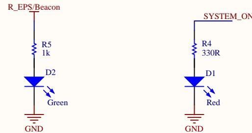
Our leds system has two leds: one green, connected to a 1k resistor, and with the R\_EPS/Beacon alimentation. The other led is red, and is connected to a 330 ohms resistor and to the SYSTEM\_ON signal. When our system is not receiving any signal, the red led will shine. If we have signal, then this will turn off, and the green one will shine.
