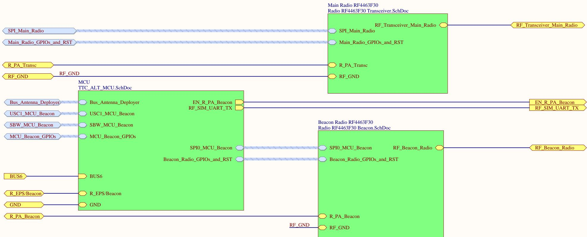
We observe the microcontroller scheme and the two RF modules that we will use, as well as the connections already explained above. The antenna module ("Beacon") is connected directly to the microcontroller, while the transmitter module ("Transceiver") is not connected to the microcontroller. The following schematics will explain both the microcontroller and the RF modules, as well as the electronics needed to work.
