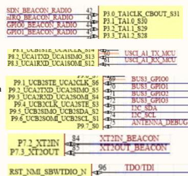
Those are the unidirectional pins. First of them is pin 13. It is an input terminal for the 32'768 kHz crystal oscillator that we will use in our design. Pin 14 is the output terminal for the same oscillator. The last pin that
