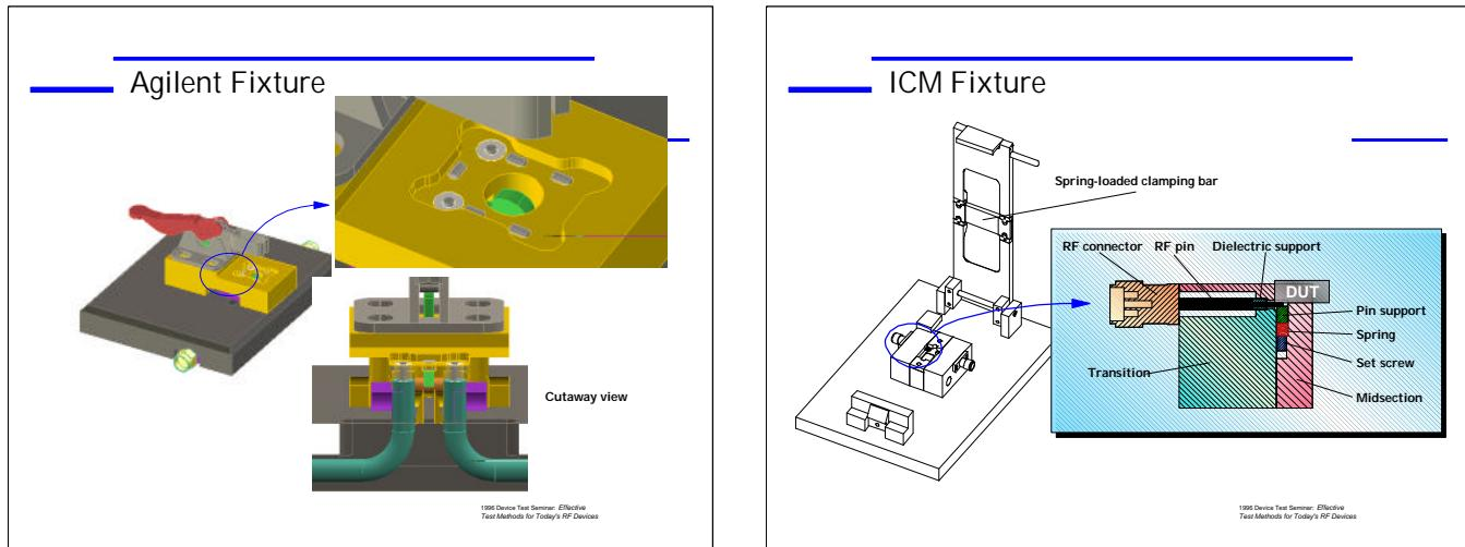
One of the most challenging aspects of fixture design is to provide a good RF path between the test cables and the DUT. The goal is to maintain  $Z_0$  (usually 50 ohms) across different transmission line media, while minimizing reflections at discontinuities.
