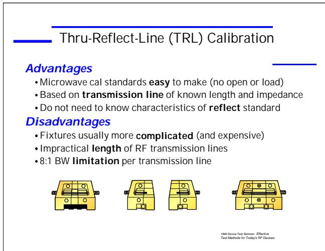
Now that we have looked at the various aspects of making good RF fixtures, let's examine our error-correction choices. The relative performance of our fixture compared to the specifications of the DUT will determine what level of calibration is required to meet the necessary measurement accuracy.
