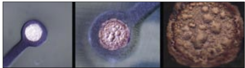
Figure 8 - The two SEM images show the surface of the 0.020" 0.5mm capture pad (left) after separation from the bottom of the 0.010" 0.25mm blind via (right). There is no evidence of a fractured surface suggesting that a true bond could not have formed during the blind via plating process. Although no measurement of the force to remove the capture pad has been made, the bond was noticeably weaker than pads of the same size on known good vias
